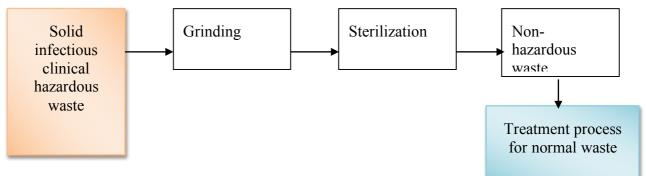
This treatment technology is one modern technology which has all processes for thorough treatment of all infectious clinical hazardous wastes, can be used for treatment of different types of solid clinical wastes including sharp items and can remove most of pathogens from the wastes.
