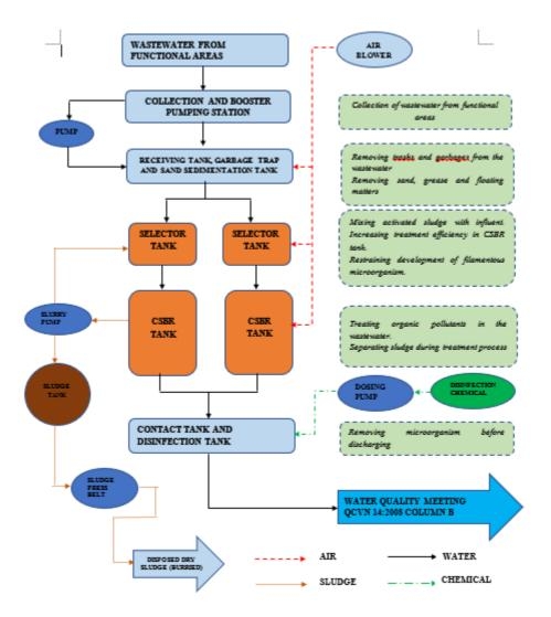
Figure 1.4: WWTP 2 Wastewater Treatment Process
