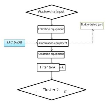
Figure 1.3: Laboratory Wastewater Treatment Process
